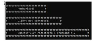
You can then close the client and your browser tab. Then, run "startapp.bat". After a while you should see two windows, one is the Alexa client and another is the python bridge, which is used to connect the client with Unity. These need to be kept open while running the unity client.
