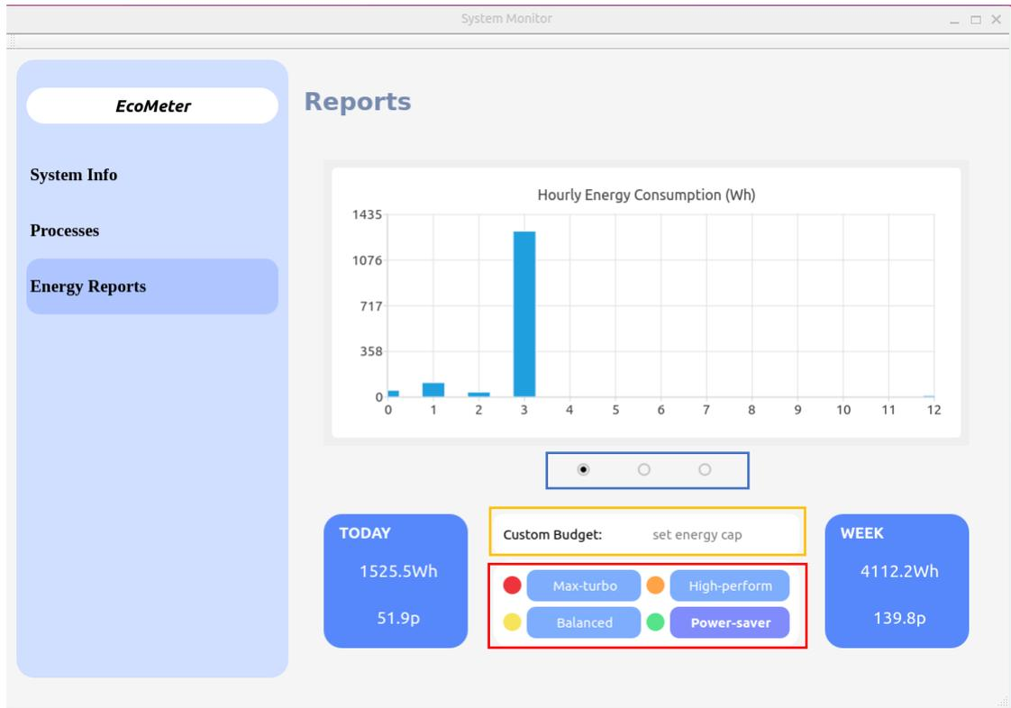
Currently, it shows the 'Energy report' interface, which allows users to view energy usage in different charts. Users can also see the total amount of energy used today and this week and the corresponding price, and set budget. Users can also switch between different power modes of this computer.
