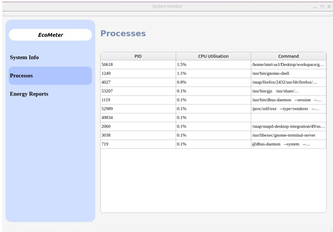
Currently, it shows the 'Processes' screen, where you can see the processes currently underway on the computer, as well as their PID, CPU utilisation and Command.
