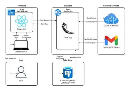
This diagram illustrates a high-level system architecture which represents how the project will be deployed
